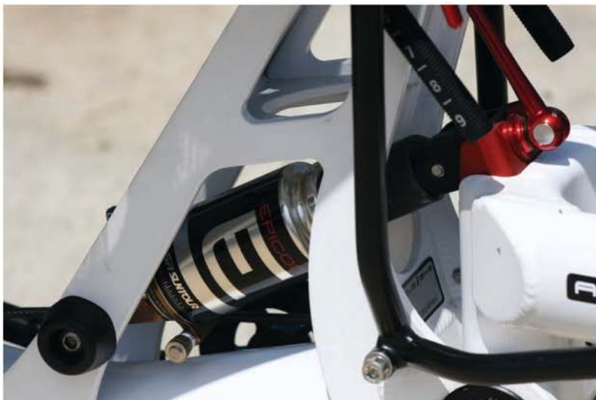
Above: Our test trike was fitted with the optional Suntour Epicon air shock with a lock-out feature.
