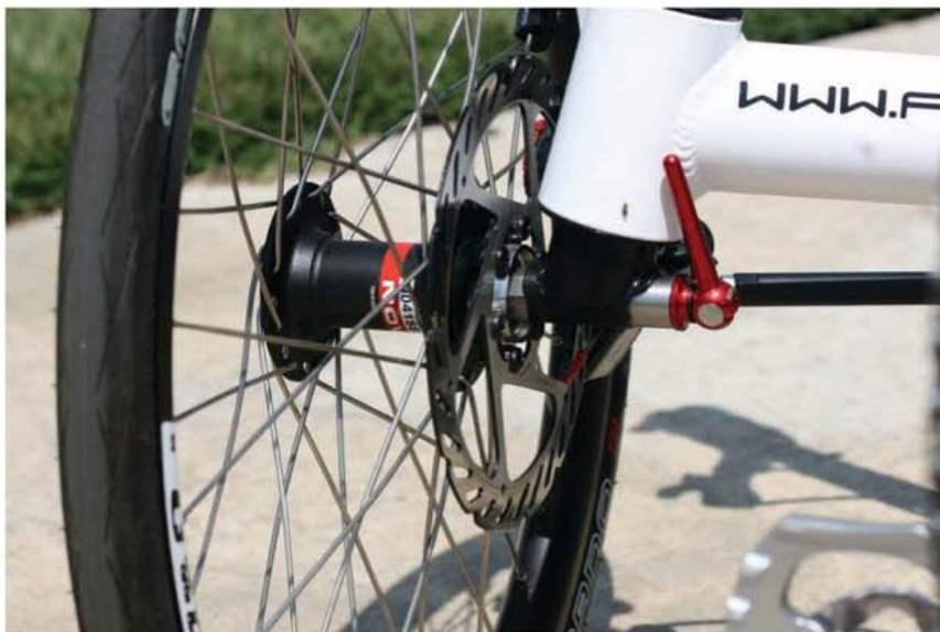
Below: Quick-release levers allow easy removal and installation of the two front wheels.
