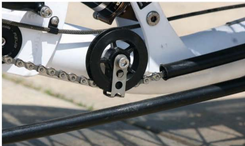
Above: Chain management includes plastic tube run for nearly the entire length of the chain and a sturdy-looking idler pulley on the return stretch of chain.
