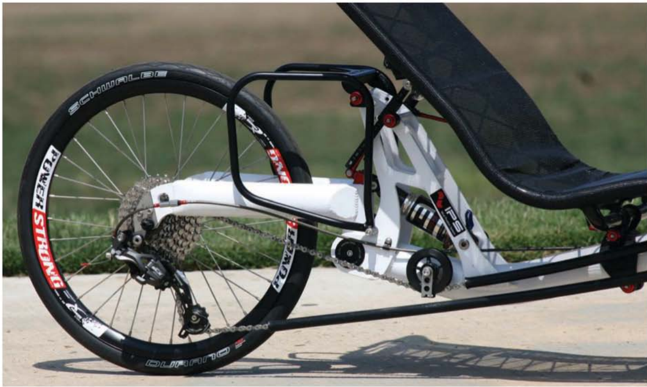
Above: Running gear includes Schwalbe Durano 1.1" tires on Remerx Total Strong 6083 aluminum 406-18 rims with Novatec hubs in front and an AZUB hub in the rear. All three wheels are fitted with 36 stainless steel spokes. Below: The seat can be adjusted fore/aft, and the trike is equipped with an adjustable boom, so a large range of adjustment allows the bike to 'customize' to a perfect fit.
