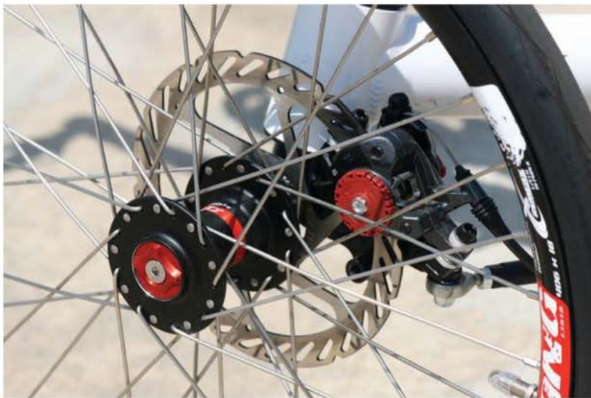
Above: Dependable, well-modulated braking power comes from a pair of Avid BB7 mechanical disk brakes, each brake includes a parking feature.
