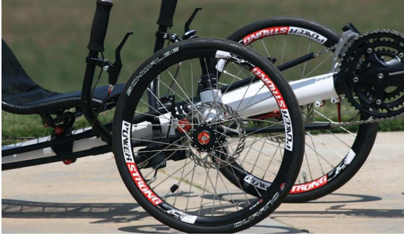
Above: Running gear includes Schwalbe Durano 1.1" tires on Remerx Total Strong 6083 aluminum 406-18 rims with Novatec hubs in front and an AZUB hub in the rear. All three wheels are fitted with 36 stainless steel spokes. Below: The seat can be adjusted fore/aft, and the trike is equipped with an adjustable boom, so a large range of adjustment allows the bike to 'customize' to a perfect fit.
