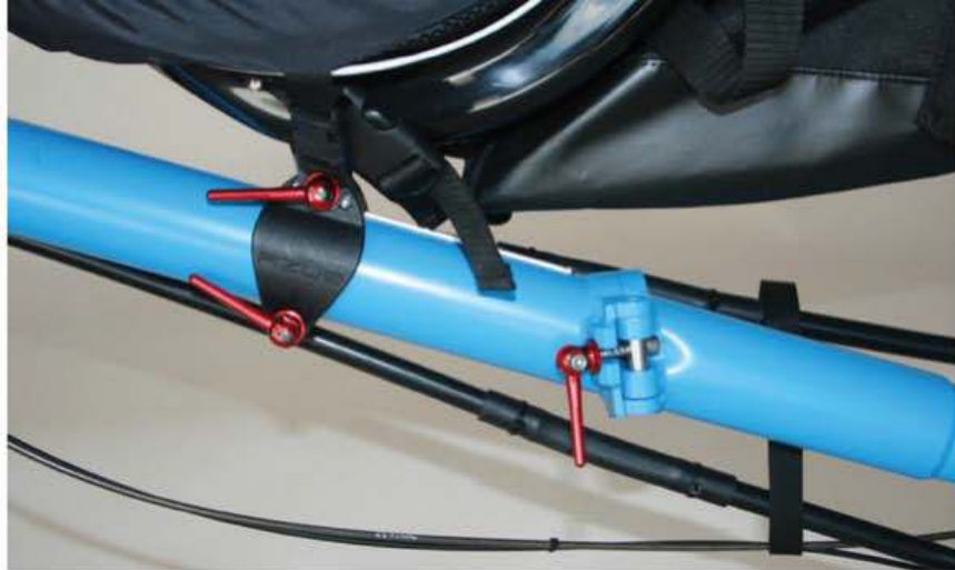
The dual quick releases on the left allow for adjusting the seat. The single QR on the right allows the Origami's frame to be quickly and easily folded for storage or travel. Multi-step unlocking process guards against accidental release.
