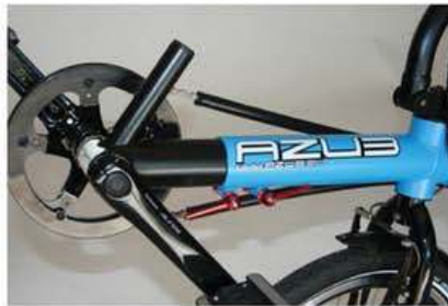
Above left: The bike's boom tube is easily adjustable. Our test unit was equipped with a rear derailleur spring setup, allowing boom-length adjustments without the need to add or remove chain links.
