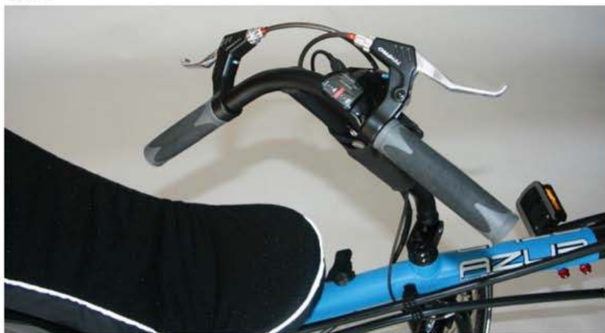
Above and below: The Origami's handlebars and controls were a fine fit for our tester. Handlebar height is adjustable, as is the fore/aft positioning. Bar tilts full-forward to ease mounting and dismounting the bike.
