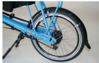
Out test Origami was fitted with an 8-speed Shimano Alfine internally-geared hub. Chain tensioner can be seen on the right side of the wheel assembly. Other multi-gear hubs, such as the popular and reliable 14-speed Rohloff Speedhub 400/14 can also be fitted when ordering a new Origami.
