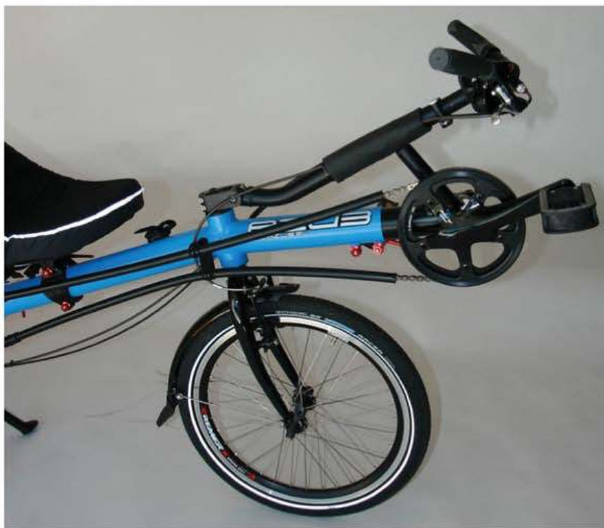
Above and below: The Origami's handlebars and controls were a fine fit for our tester. Handlebar height is adjustable, as is the fore/aft positioning. Bar tilts full-forward to ease mounting and dismounting the bike.
